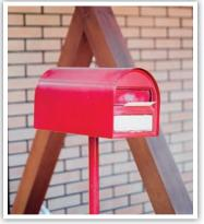
winter hazard and the Town will not repair or replace the mailbox or post. The height of the bottom of the mailbox to the street should be between 42"- 48" and the mailbox door should be 6 to 8 inches back from the front face of the curb or road edge.
